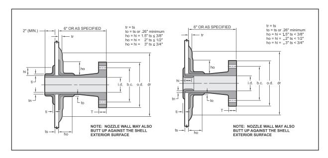
Actual installation may be either flush or penetrating, with inside welds seamed in accordance with ASME RTP-1, and as shown above. Bolt holes shall straddle the natural centerline of the tank, unless otherwise specified.
