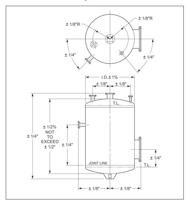
6.2 **Body Flanges:** Body flanges shall be flat and true to a required tolerance as follows: flanges less than or equal to 84" diameter, true to +1/32", flanges over 84" through 108" diameter, true to +1/8", and flanges over 108" diameter, true to +3/32".
